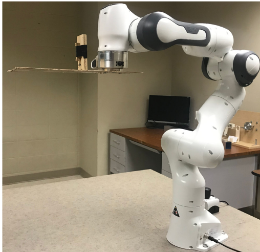
Fig. 8. Experimental setup with an object to manipulated placed on top of a tray, which is mounted to the end effector of a robotic manipulator.
