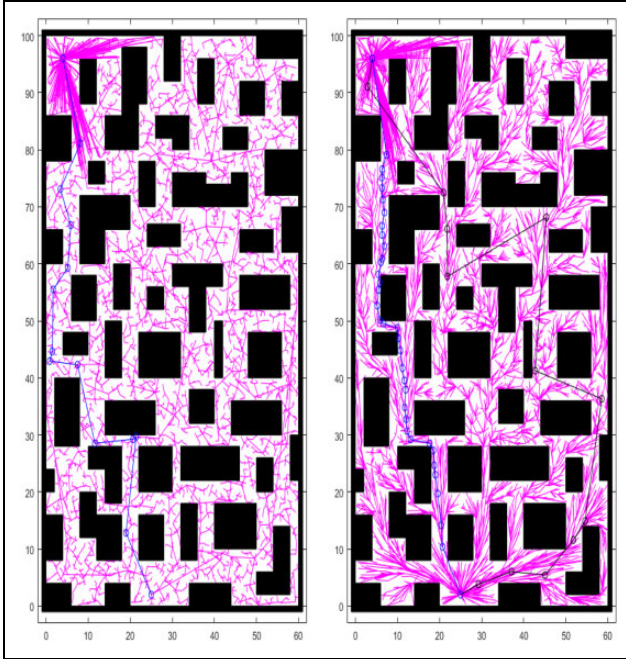
Figure 1. Results of RRT (left) and RRT* (right) with 5000 nodes. The blue line represents the best path found and the black line represents the first path found by the RRT. RRT: rapidly exploring random tree; RRT*: extended rapidly exploring random tree.
