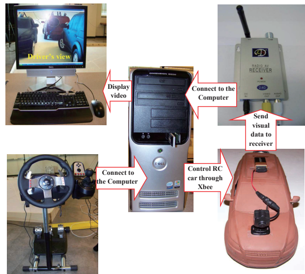
Fig. 3. The setup for manually driving the RC car.
