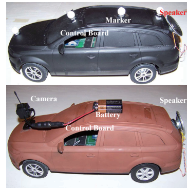
Fig. 2. Two RC car platforms: (Top) for automatic driving control, (Bottom) for manually driving control.
