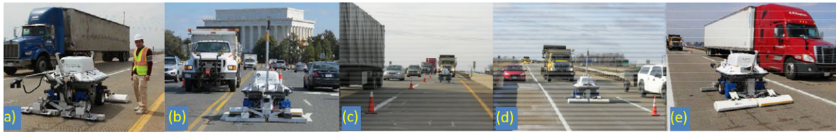
FIGURE 14 Deployment of the NDE robot for inspection of more than 40 bridges: (a) Inspect the Chicago Mile-long bridge in Illinois April 2014 (the co-author Hung La with the robot in this picture); (b) Inspect the Arlington Memorial Bridge in DC, April 2014; (c) Inspect the Haymarket highway bridge in Virginia, May 2014; (d) Inspect the Ogden Avenue Bridge, Downers Grove, Illinois, December 2014; (e) Inspect the Chicago Avenue Bridge in Dixon, Illinois in April 2014
