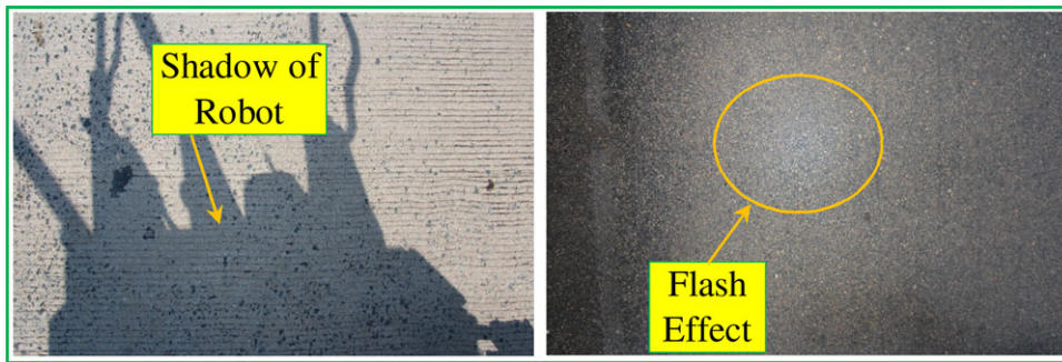
FIGURE 8 (Left) Shadow problem with day time image collection. (Right) Flash light effect at night time image collection
