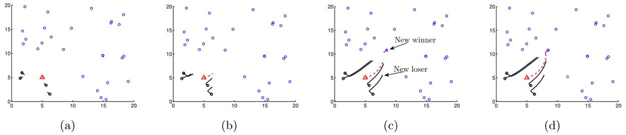
**Fig. 2.** Snapshots for moving target tracking and the corresponding tracking trajectories, where initial locations of mobile robots and the moving target are randomly generated. (a) Snapshots at  $t = 0.3$  s. (b) Snapshots at  $t = 1.7$  s. (c) Snapshots at  $t = 2.5$  s. (d) Actual path of the moving target and tracking trajectories of different mobile robots.
