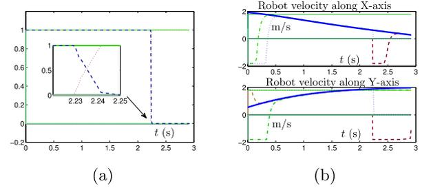
**Fig. 3.** Outputs of  $k$ -WTA network and the corresponding velocities of mobile robots at different phases. (a) Outputs of  $k$ -WTA network. (b) Velocity profiles of mobile robots with blue lines denoting the velocity profiles of the moving target. (For interpretation of the references to color in this figure legend, the reader is referred to the web version of this article.)
