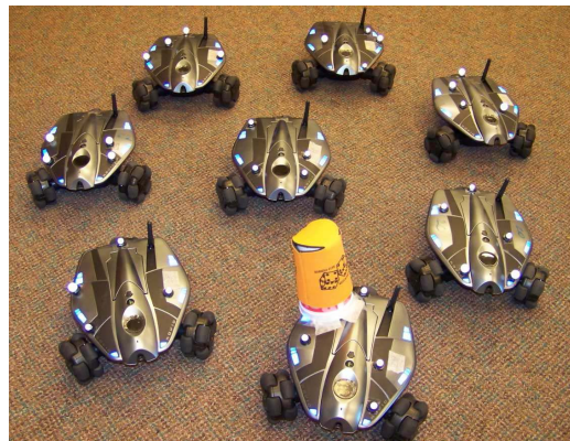
Fig. 12. Seven Rovio prey robots and one Rovio predator robot (marked with a yellow cup) are used in the experiment.
