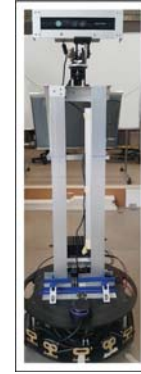
Fig. 2. Experiment platform equipped with Microsoft Kinect and RPLIDAR-A3 laser range finder.
