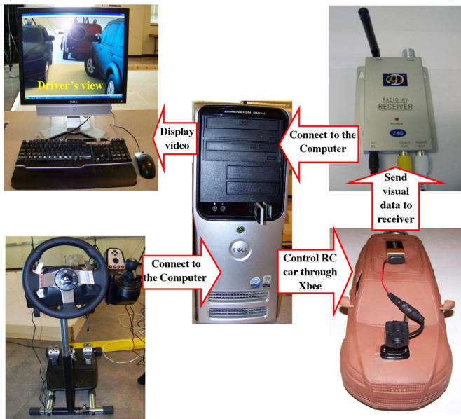
Fig. 3. Setup for manually driving RC cars.
