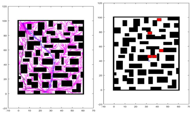
(a) Search tree and robot path. (b) Moving obstacles block the path.
