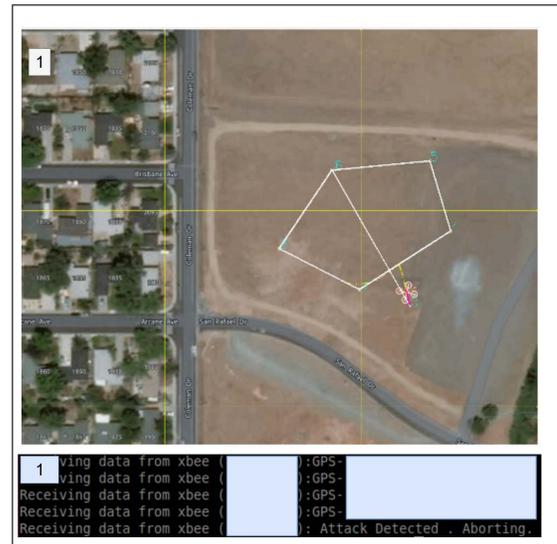
Fig. 5. Waypoints set for the experiment in the first configuration. The attack was discovered after the UAV navigated from waypoint 3 and Return-to-Launch (RTL) was enabled.
