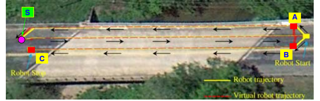
Fig. 6. Schematic of motion planning of the inspection robot on a bridge (the picture shown here is the top view of the Pohatcong Creek Bridge near the township of Bloomsbury, Warren county, New Jersey, USA.)
