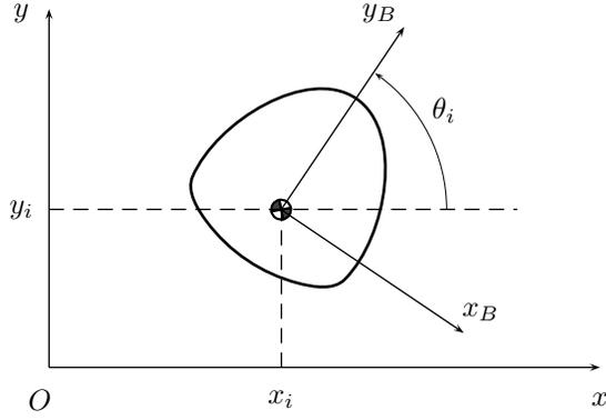
Fig. 1. Configuration of the  $i$ -th mobile robot.
