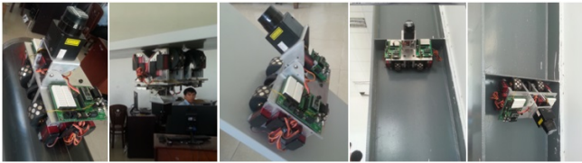
Fig. 15. Robot can adhere to steel surfaces in different situations.
