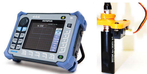
Fig. 3: (Left) Industrial Eddy current sensor Nortec 600; (Right) sensor probe for data collection.
