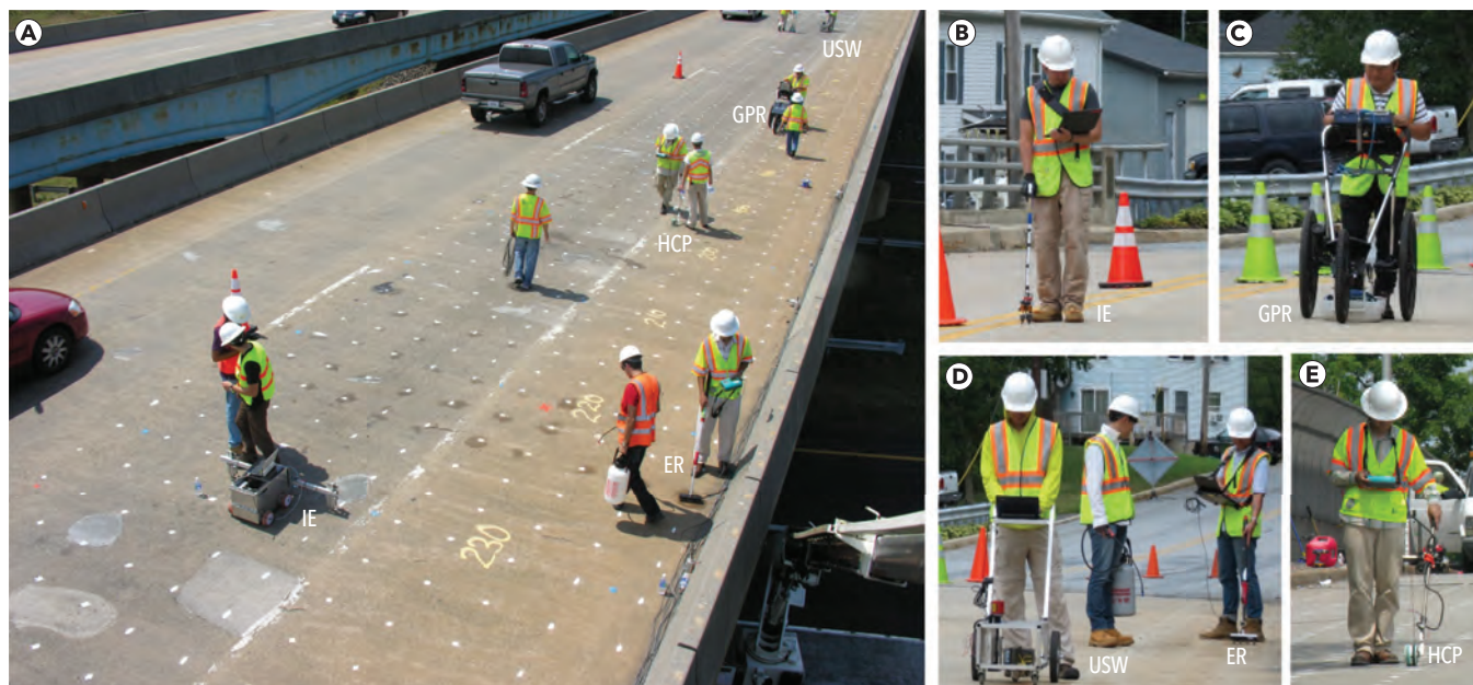
Figure 1. Manual NDE data collection on a bridge deck (a) using the following NDE technologies: (b) impact echo; (IE); (c) ground penetrating radar (GPR); (d) ultrasonic surface waves (USW) and electrical resistivity (ER); (e) half-cell potential (HCP).
