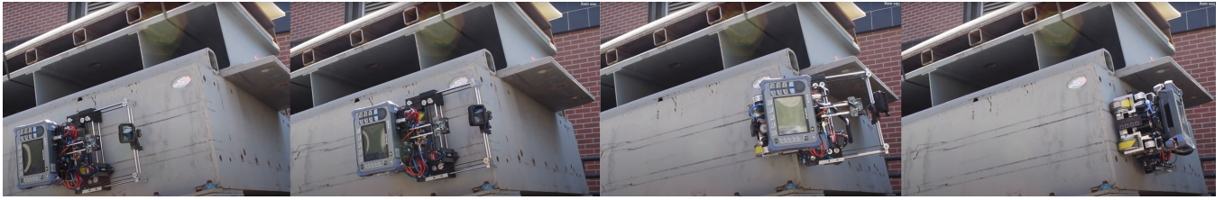
Fig. 11: Robot testing on flat steel structures and passing external corner.
