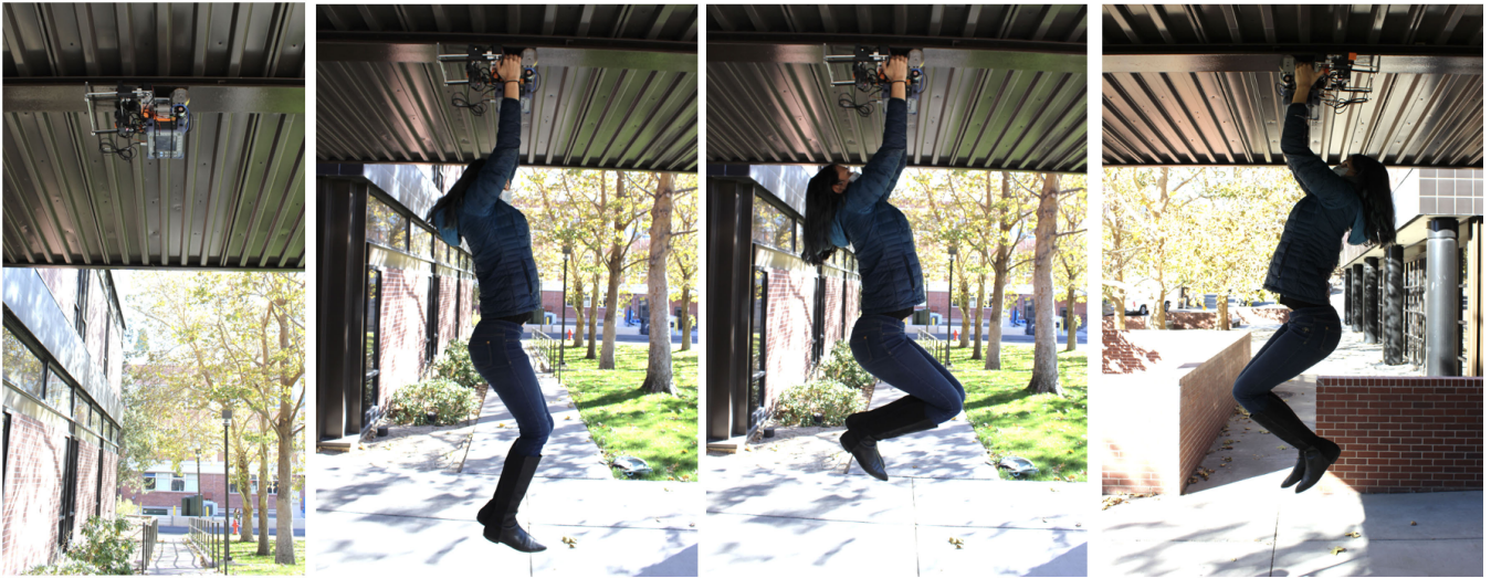
Fig. 8: Adhesion test: a woman (weight of 64kg) hanging from robot adhered to steel I beam. The robot's adhesion force is significantly stronger than the force that multiple people can exert combined is.
