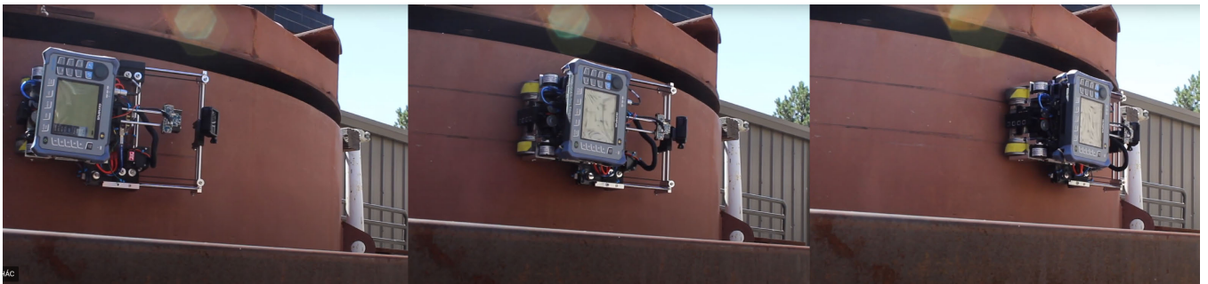
Fig. 9: Robot testing on a curved steel surface.
