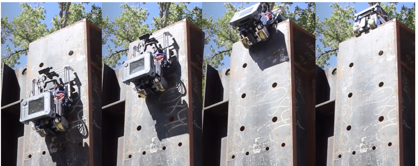
Fig. 10: Robot testing on perforated surface.
