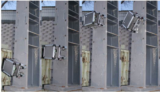
Fig. 10: The robot traveling up a steel beam using each of the steering methods from left to right.
