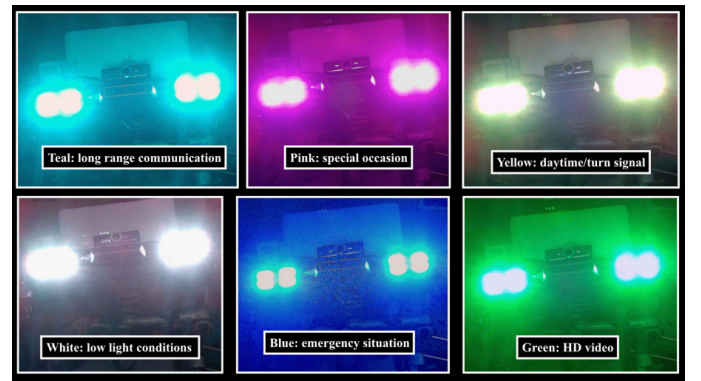
Fig. 5. iChair LED color options and their operation is followed by Algorithm 1. These lights are not just for show, even though being seen is vital when attempting to avoid collisions. With 7 color, 10 pattern, and 5 different speed options we can enhance observations and communicate over long distance.
