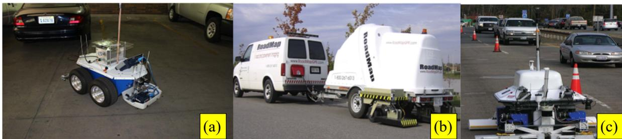
**Figure 1: Some of the state-of-the-art robotic platforms employing a wide-range of sensors for infrastructural monitoring (a) NDE robotic platform (Gibb et al., 2017), (b) Roadmap system (Diamanti and Redman, 2012) and (c). RABIT platform (La et al., 2017)**
